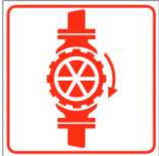
Sprinkler Stop Valve
