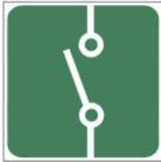
Electric Isolator Switch
