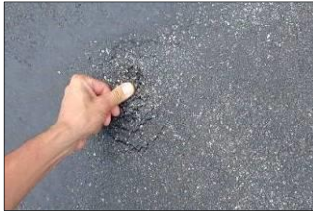
Figure 13. Sensitivity of Geotextile Seal to Cutback Emulsion Tack Coat
