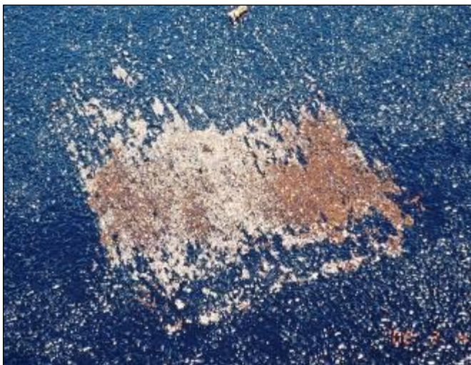
Figure 14. False Break with Modified Emulsion
