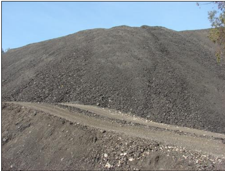
Figure 8. Reclaimed Asphalt (RA) Stockpile
